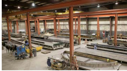
Image 4.2, Precast Concrete Forms
